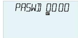
Through the password to limit the right of customers to set some important parameters, and four digitals are required to enter, default password is "0000".
