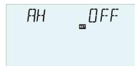
▶ Press “SET” button, “AH OFF” blinks on the screen
