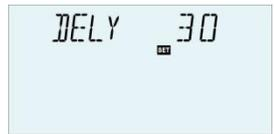
▶ Press “↑”, “↓” button, to adjust the delay detect time when no flow
