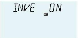
▶ Press “↑”, “↓” button, to activate this function, “INVE ON” displays on the screen
